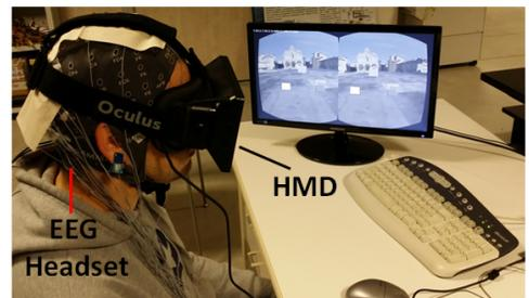
Fig. 5. The experimental setup used to validate the proposed SSVEP-BCI approach based on CNN classification.
