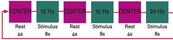
Fig. 6. The logical scheme of the training phase. Each trial is composed by three phase of rest (in violet) and visual stimulation (in green).
